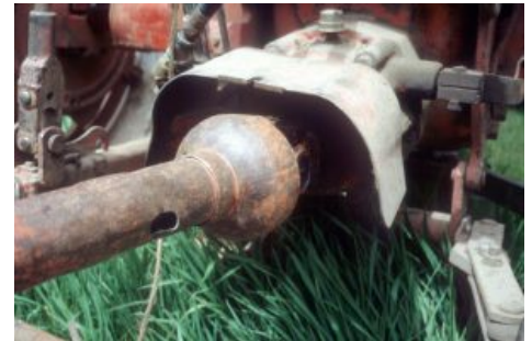
The PTO master-shield covers a common area of entanglement and injury. Photo credit: John Shutske
